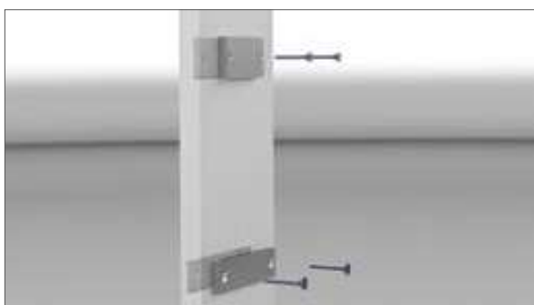
Fix base plate at the basic substructure
