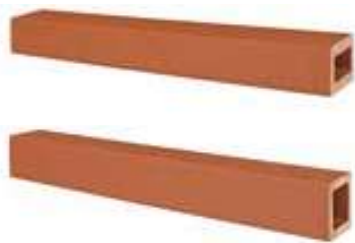
Rectangular tube 50 x 60 mm / 60 x 60 mm Work size: 50 x 60 mm / 60 x 60 mm Weight: 50 x 60 mm: 4.29 kg / lin. m. 60 x 60 mm: 4.49 kg / lin. m. available unglazed as well as with 4 glazed sides. Possible up to a length of 1,800 mm on request
