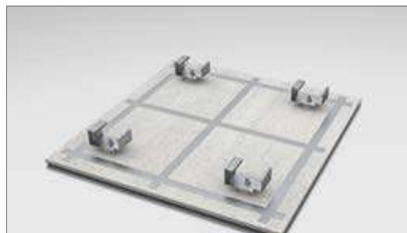
Screw clasps with rubber washer (Art. no. 371) and stainless steel nut (Art. no. 370) on the Quadro fastening points on the reverse side of the panels
